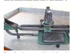
The cradle and support assemble tracks forward and aft along dual rails to adjust for firearms of different length and design.
